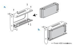
• Mount the bracket to the computer case and secure it with the screw from the PC.
