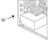
• After the hardware install, connect your SATA and Power cable (not included) to the HDD and power supply. Then you can start using it.
