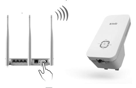
2. Press the RE button on the wireless range extender for 1~3 seconds within 2 minutes;
