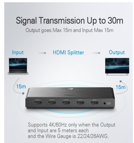
Signal Transmission Up to 30m
