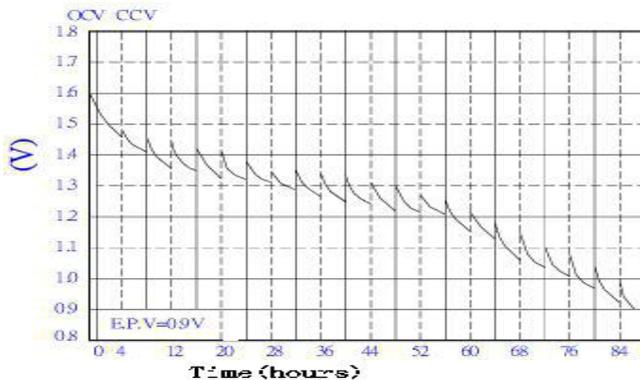
Test Condition: Load Resistor 43Ω, 4h/d, 20°C±2°C and 60±15%RH
