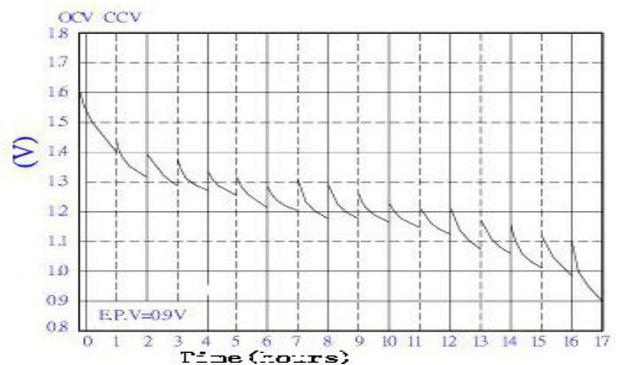
Test Condition: Load Resistor 10Ω, 1h/d, 20°C±2°C and 60±15%RH
