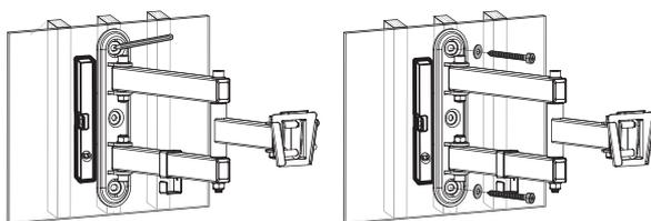
Install the wall plate to the wall
