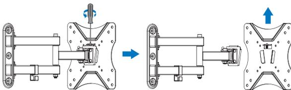
Remove the wall plate from the wall mount
