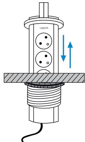
Tighten the detachable locking ring clockwise from the bottom of the socket.
